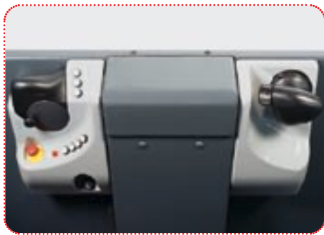
Control Panel arrangement for operation in travel direction load.
