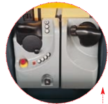
Control Panel arrangement for operation in travel direction mast.
