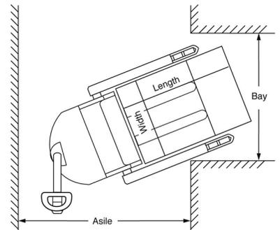
Aisle dimensions listed above assume the minimum bay width to be straddle OD plus 5" (2.5" on each either side of straddle leg). Straddle OD is the load width plus 10". Truck performance may vary due to application requirements and changes in model design.
